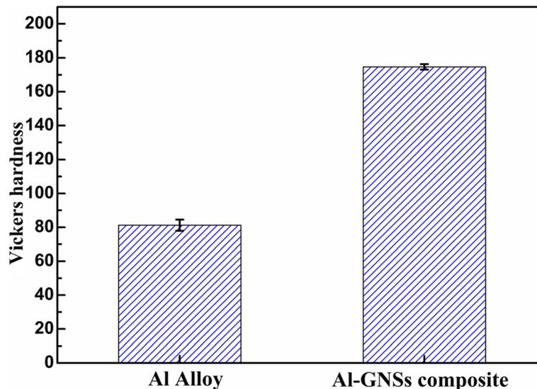
**Fig. 10** The mean Vickers hardness of the synthesized Al alloy and Al-GNSs bulk materials
