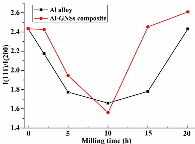
**Fig. 6** The intensity ratio of (111) to (200) at different milling times
