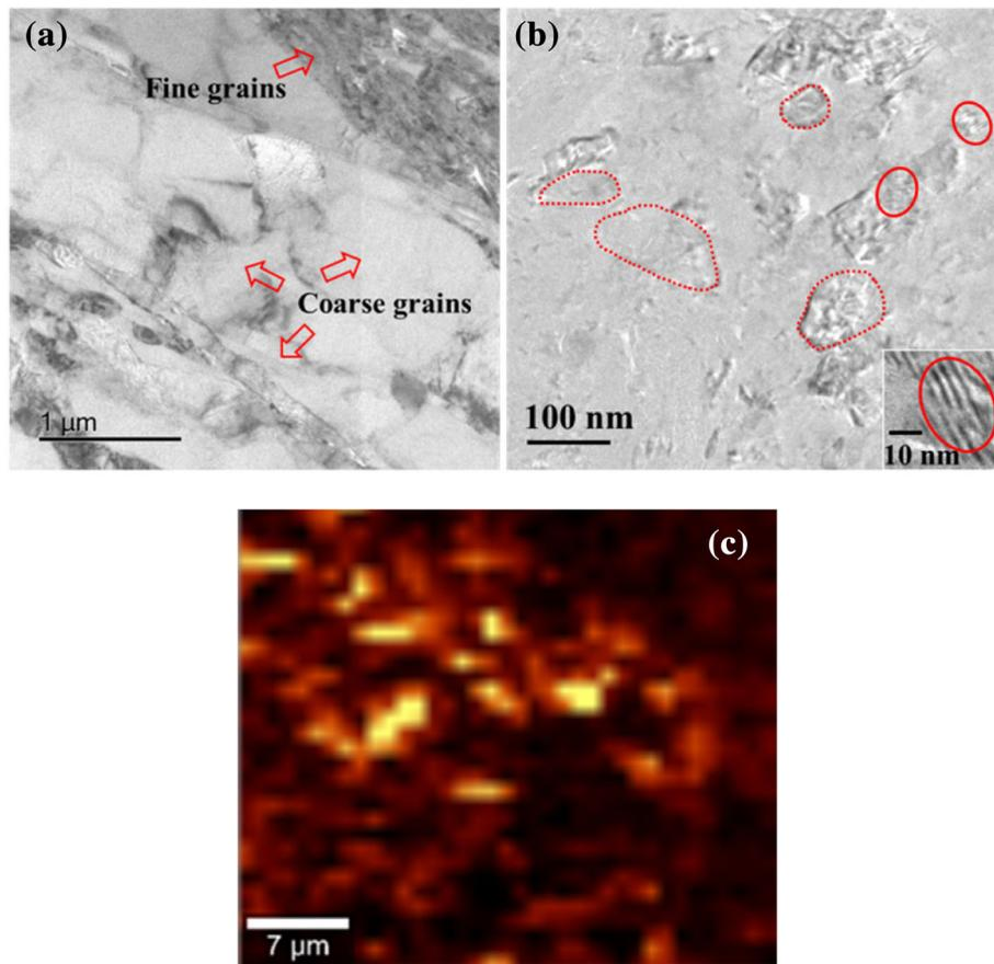
**Fig. 9** TEM micrographs of the produced (a) Al alloy, and (b) Al-GNSs composite. Grains are indicated using dashed circles; highly deformed regions are marked using solid circles. **c** The Raman mapping of G band on the Al-GNSs composite
