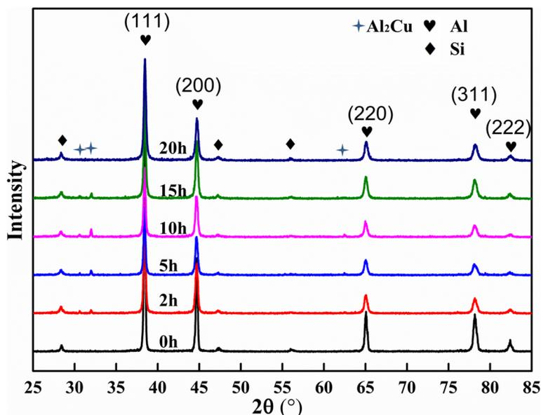
**Fig. 4** The XRD patterns of the ball milled Al alloy powders at different times
