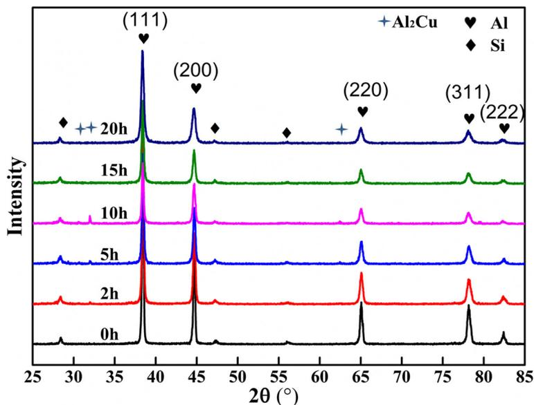
**Fig. 5** X-Ray diffraction patterns of the ball milled Al-GNSs composite powders at different times
