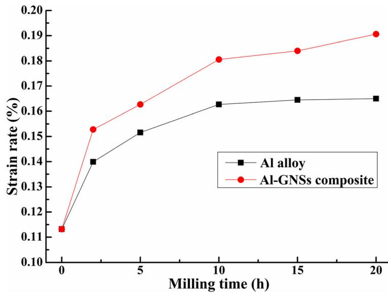
**Fig. 8** The evolution of lattice strain for Al alloy and Al-GNSs powder mixtures at different milling times
