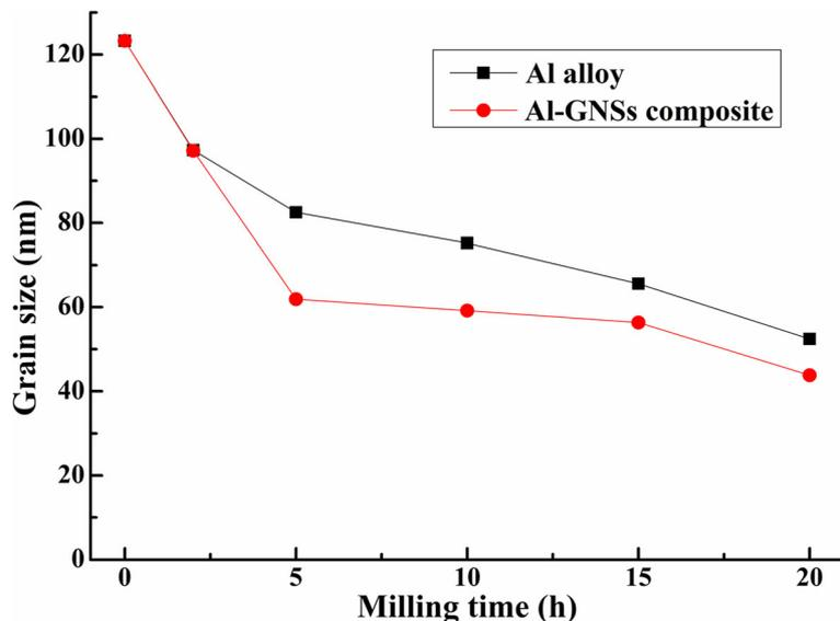
**Fig. 7** The evolution of crystalline size for Al alloy and Al-GNSs powder mixtures at different milling times
