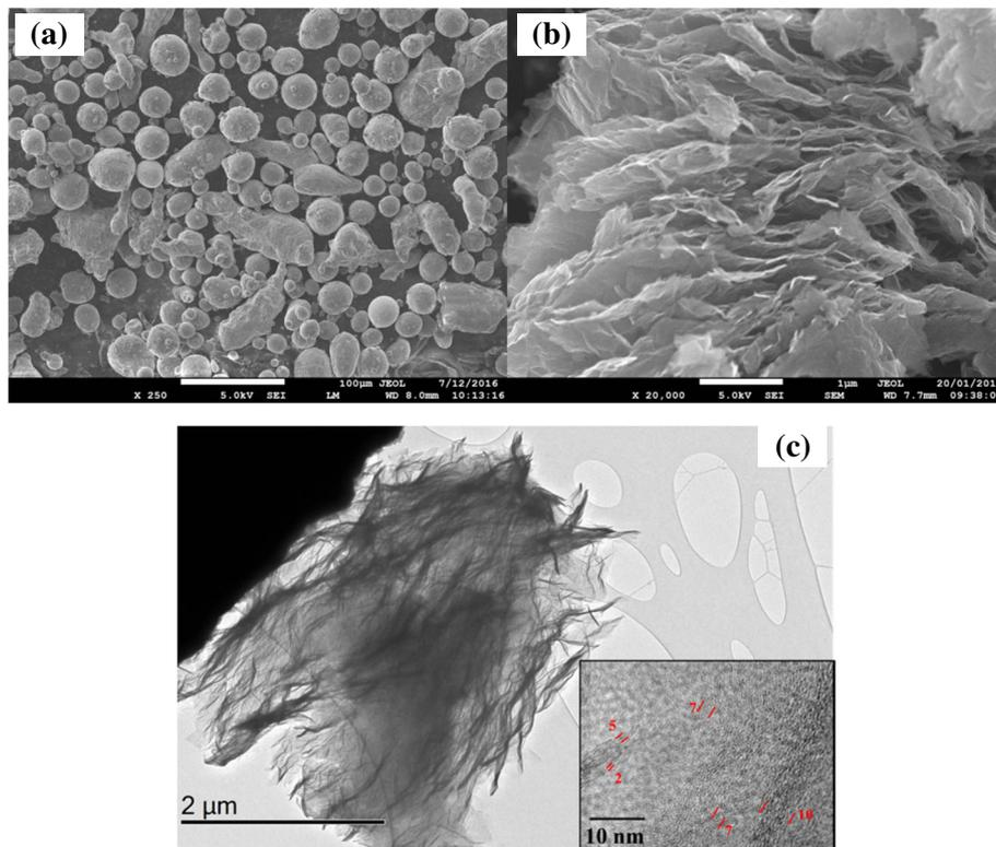
**Fig. 1** The SEM morphologies of the as-received (a) aluminium powder. The morphology of the as-received GNSs observed using (b) SEM and (c) TEM. The inset shows a high-resolution micrograph of the lattice of the GNSs, with indicated number of layers
