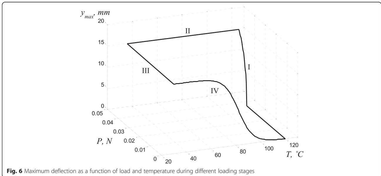
**Fig. 6** Maximum deflection as a function of load and temperature during different loading stages
