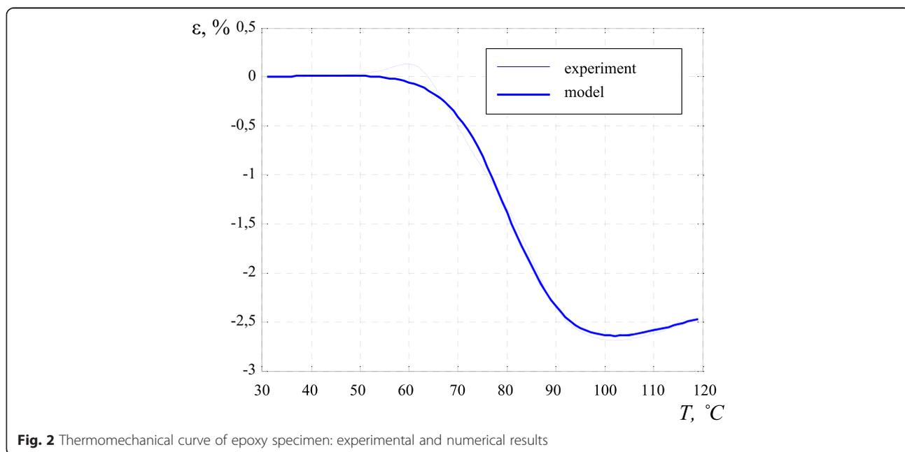
**Fig. 2** Thermomechanical curve of epoxy specimen: experimental and numerical results
