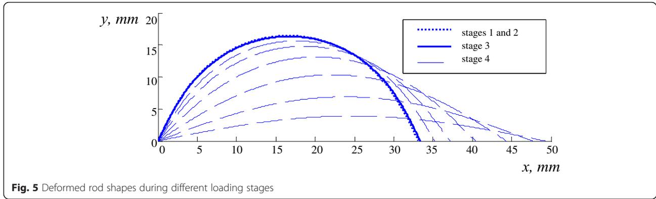
**Fig. 5** Deformed rod shapes during different loading stages
