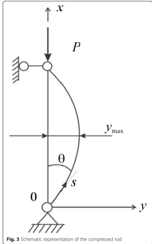
Fig. 3 Schematic representation of the compressed rod
