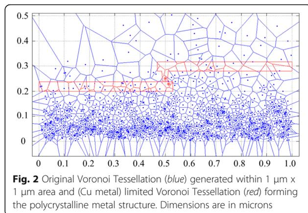
lognormally distributed pseudorandom points for the y-coordinates (vertical). With this approach we obtain smaller grains at the bottom and larger grains at the top as shown in Figs. 2 and 4. The grains with diameter less than 6 nm were merged with adjacent grains to account for smaller grains being consumed by the adjacent larger grains during grain growth. The lognormal probability plot of the grain size distribution obtained by Voronoi tessellation is shown in Fig. 3.
