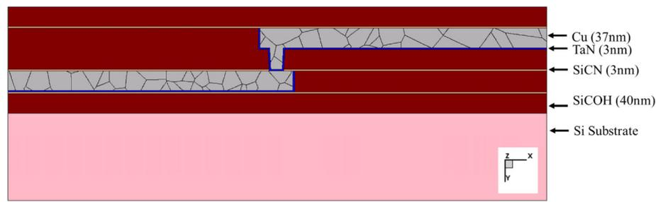
**Fig. 4** Cross section of polycrystalline test structure created using Cu metal boundary limited Voronoi tessellation to form the polycrystalline Cu metal structure
