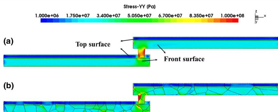
**Fig. 5** YY component of node stress levels obtained post the thermal stress: **a** crystalline Cu metal structure with isotropic elastic constants and **b** polycrystalline Cu with grain orientation dependent elastic anisotropy. (Note that this is a tilted view of a 3D structure, showing only stress levels in copper while hiding other materials in test structures)
