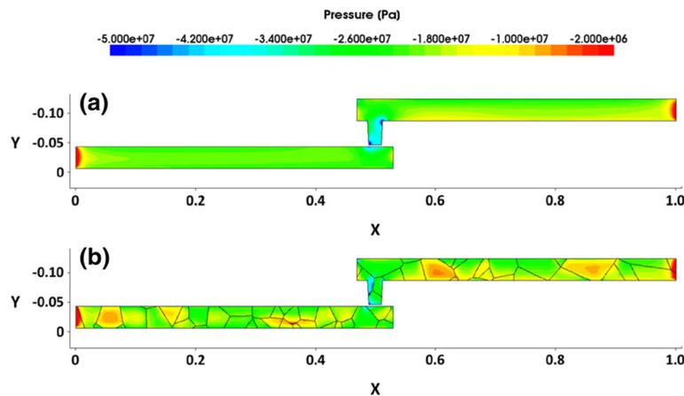
**Fig. 8** Cross section of test structures showing pressure levels obtained post the thermal stress: **a** crystalline Cu metal structure with isotropic elastic constants and **b** polycrystalline Cu with grain orientation dependent elastic anisotropy
