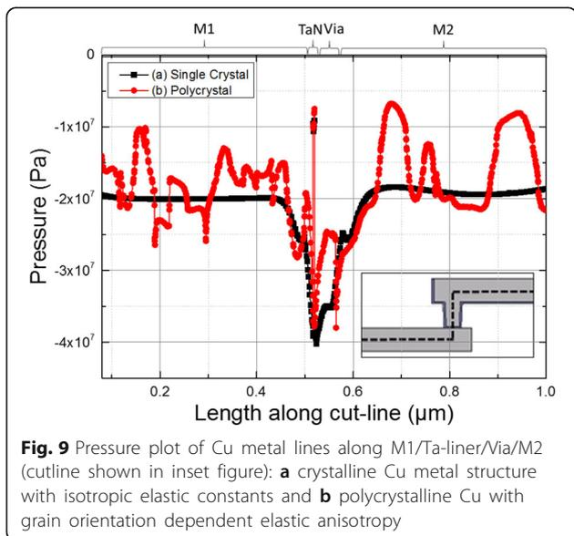
**Fig. 9** Pressure plot of Cu metal lines along M1/Ta-liner/Via/M2 (cutline shown in inset figure): **a** crystalline Cu metal structure with isotropic elastic constants and **b** polycrystalline Cu with grain orientation dependent elastic anisotropy
