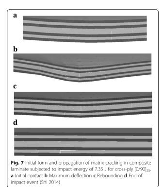
elements, especially in angled ply, well captured the matrix cracking and splitting.
