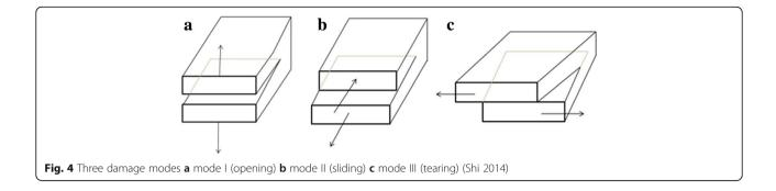
values between zero and one. When  $\xi = 0$  the crack was mode I driven, while as  $\xi \rightarrow 1$  propagation was mode II dominated (and this could be also the case when  $\eta = 0$ ).
